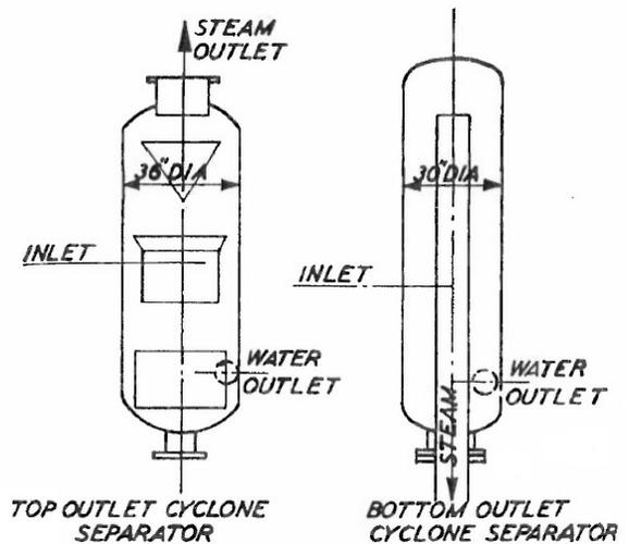
Figure 1. Schematic diagram of top outlet cyclone separator (TOC) and bottom outlet cyclone separator (BOC).
