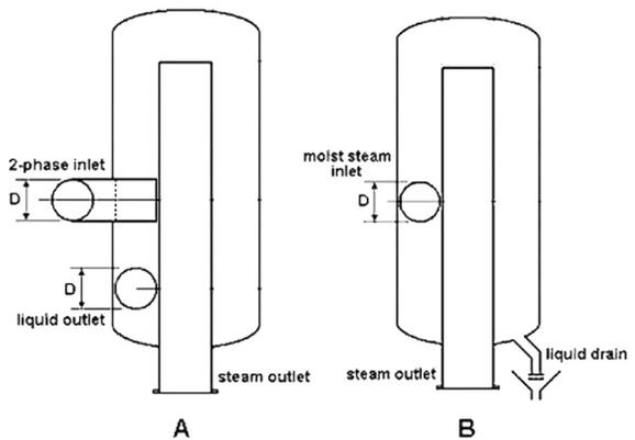
Figure 2. Schematic diagram of steam-water separator (A) and steam dryers (B).
